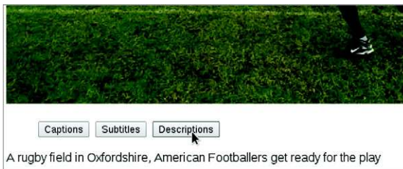
Figure I.6 JavaScript has been used to extract the text content of the normally invisible description track and display it on the screen.
