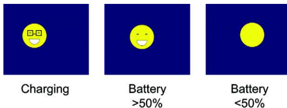
Figure I.16 By integrating the Battery API, you can make your app do less work as the charge level drops.
